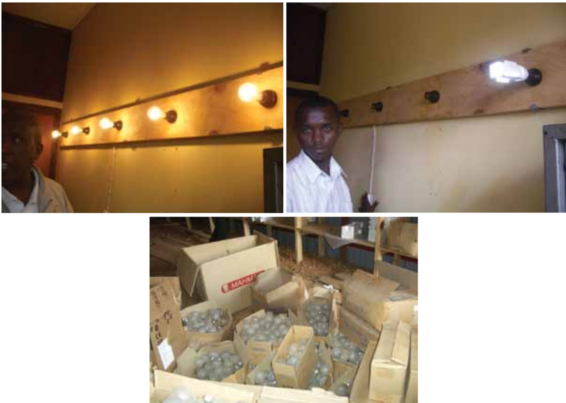
Testing of incandescent and compact fluorescent lamps at Electrogaz center in Rwanda. [When a customer returns incandescent lamps and buys CFLs, a project requirement is that both types of lighting be tested. This ensures the replacement of functioning incandescent lamps.]
