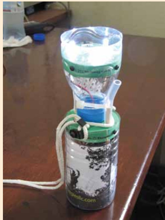
A taa bora made from a recycled plastic water bottle, rechargeable AA batteries, and an LED bulb. With a slight modification, it doubles as a desk lamp for studying.
